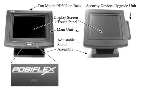
The security device and top mount LCD customer display are options to both 12" and 15" models. The LED in the logo area serves for several purposes through giving different indication of steady/flashing green/blue light. Please refer to the paragraph discussing the LED indication in the chapter of "USING THE TOUCH POS" of this manual.
